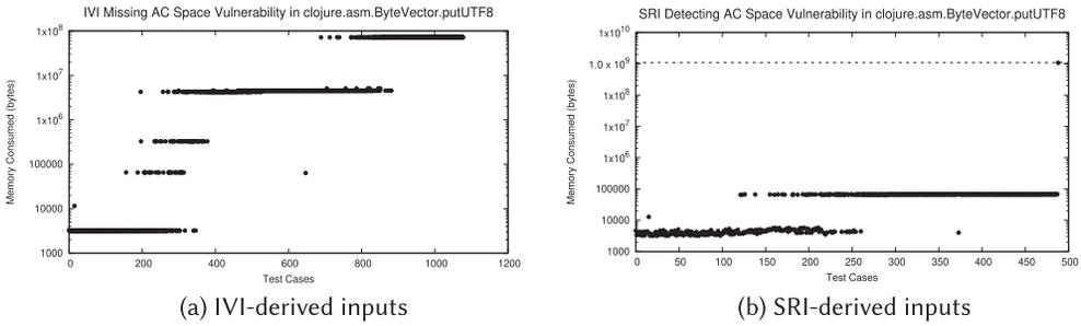
Fig. 10. Micro-fuzzing `clojure.asm.ByteVector.putUTF8` with IVI-derived inputs fails to detect a zero-day AC vulnerability in the Clojure runtime, while SRI-derived inputs detect the vulnerability using fewer test cases (see the upper-right-hand corner of Graph (b)). Note that the y-axis for Graph (a) is 1 order of magnitude smaller than Graph (b).
