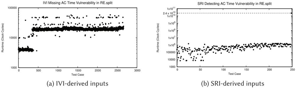
Fig. 6. Micro-fuzzing `com.sun.org.apache.regexp.internal.RE.split(String input)` with IVI-derived inputs fails to detect a zero-day AC vulnerability in the JRE, while SRI-derived inputs detect the vulnerability correctly (see the upper-right-hand corner of Graph (b)). Observe that the  $y$ -axis for Graph (a) is 5 orders of magnitude smaller than Graph (b).
