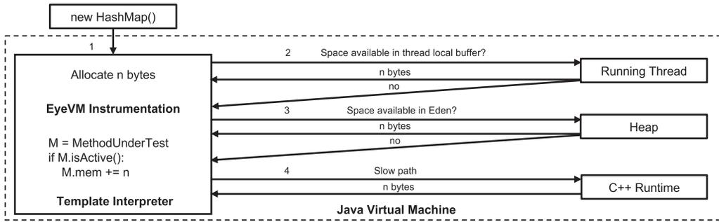
Fig. 3. The different ways the JVM may allocate an object, and how the EyeVM tracks memory usage.
