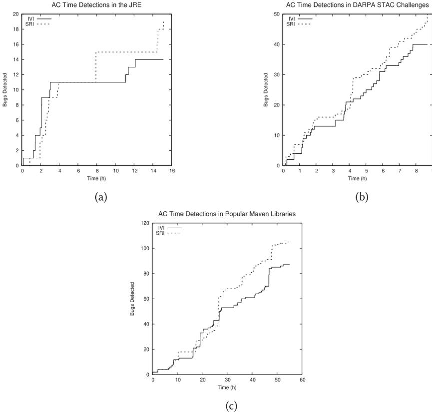
Fig. 4. Micro-fuzzing for AC time vulnerabilities with SRI-derived seed inputs outperforms IVI-derived seed inputs for the JRE (Graph (a)), the DARPA STAC program (Graph (b)), and the 100 most popular Maven libraries (Graph (c)).
