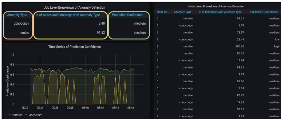
**Fig. 2.** An example SWFFT application run with the *membw* anomaly. We provide diagnosed anomaly types (orange box) and their percentage across all windows (yellow box) as well as model’s prediction confidences (green box) in the job-level breakdown. The time series plot shows the average confidence level of each anomaly across all the compute nodes used by the application. We also provide the node-level breakdown composed of the same analyses we provide in the job-level breakdown.
